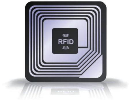
Especially with regards to the implementation of TETRA digital radio communication RFID technology is an excellent approach to meet the high requirements in logistics and administration for the supply of thousands of terminals. The typical field of application of RFID radio chips is their individual identification with regards to the logistic and administrative processing of terminals - as replacement of the typical type label.
