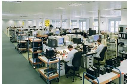
tackled. After a thorough fault analysis repairs up to component level (level 3) are carried out at SELECTRIC. For this purpose the specially skilled and continuously trained service technicians can dispose of a large pool of high-tech repair tools (e.g. infrared soldering systems).
